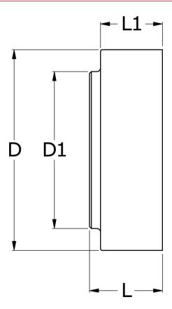
$\begin{array}{lll} D & = 440 \\ D1 & = 215 \\ L & = 180 \\ L1 & = 86 \\ Max bore & = 130 \\ Torque (N m) = 13500 \end{array}$
